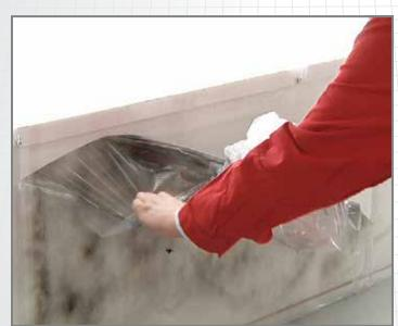
Each transparent ant-static polypropylene layer is treated with paint adhesion to trap overspray.
